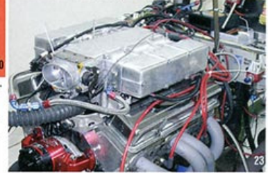
20» Somewhat of a rare find, this SLP intake came off an SLP Firehawk Firebird. 21» The cross-ram design featured a central throttle-body entry with a pair of additional plenums designed to allow the air to make the turn into the respective runners. 22» One unique feature of the SLP intake was that the fuel rails were cast into the upper manifold section. 23» The power peak was up slightly with the SLP intake, to 466 hp, while the torque peak stood at 493 lb-ft. The SLP intake was the first to start trading low-speed torque for high-rpm horsepower.
