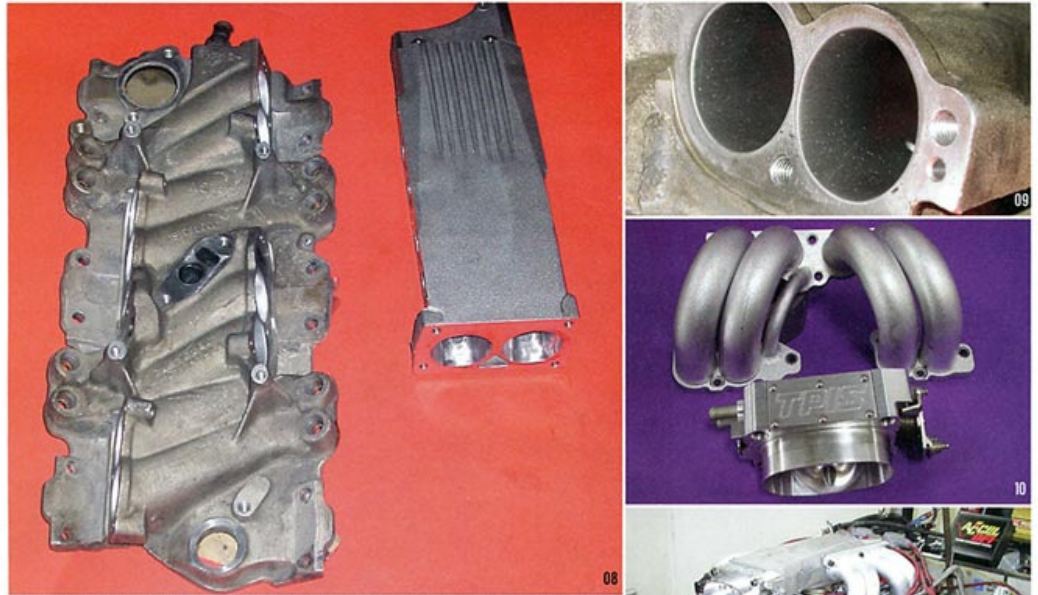
88 08 Despite their humble beginnings, the factory TPI base manifold and plenum can be made to flow better by treating them to Extrude-Hone porting. Add a set of big-tube runners (from TPIS, for instance) and you have the makings of a serious TPI system. 09 The Extrude-Hone process forces abrasive media through the ports, removing material to improve flow. The trademark wall finish is ultra smooth. The limiting factor in porting the factory base manifold is actually the size of the tubular runners. 10 We combined the Extrude-Hone ported base and plenum with a set of TPIS big-tube runners and 52mm throttle body. 11 The Extrude-Hone ported combination upped the peak power output to 451 hp, while the torque curve swelled to a whopping 534 lb-ft.
