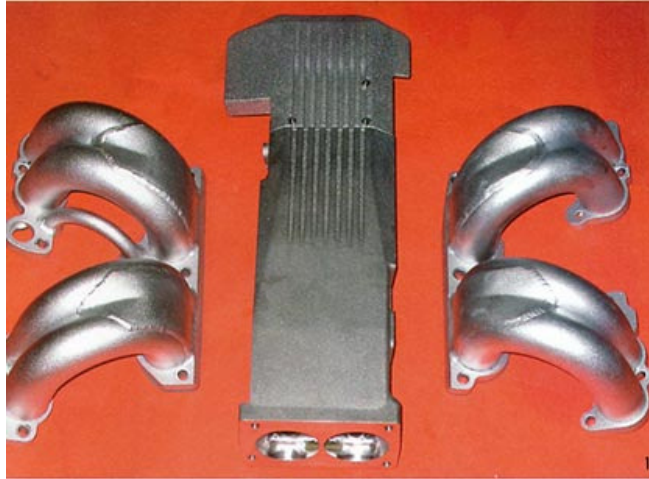
16» Arizona Speed & Marine offered up a pair of siamesed runners for testing along with a matching ported plenum. 17» The siamesed runners effectively decrease the runner length, which tends to shift the power curve higher in the rev range. 18» ASM also supplied a pair of high-flow throttle bodies for testing with its intake system—though the larger throttle body showed no gains on our test engine at the 464hp level. 19» When combined with the TPIS Big Mouth base manifold, the ASM runners, plenum and throttle body produced 464 hp, but the torque peak was off slightly to 510 lb-ft.
