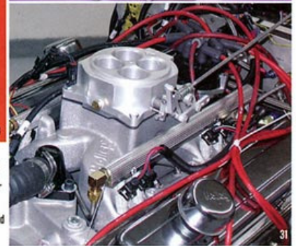
28» We were very curious to see how the Holley single-plane intake fared in this TPI test. The intake was cast for EFI use by including injector bungs, as well as a provision to attach the required fuel rails. 29» In place of the traditional four-barrel carb was a four-hole throttle body capable of flowing 1,000 cfm. 30» The Holley throttle body featured progressive linkage to improve street driveability. 31» On the dyno, the Holley EFI intake showed why so many people choose single-plane intakes for their high-performance carbureted applications, by posting peak numbers of 493 hp and 480 lb-ft of torque.
