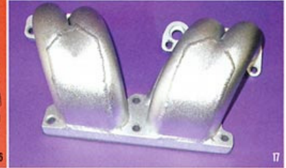
16» Arizona Speed & Marine offered up a pair of siamesed runners for testing along with a matching ported plenum. 17» The siamesed runners effectively decrease the runner length, which tends to shift the power curve higher in the rev range. 18» ASM also supplied a pair of high-flow throttle bodies for testing with its intake system—though the larger throttle body showed no gains on our test engine at the 464hp level. 19» When combined with the TPIS Big Mouth base manifold, the ASM runners, plenum and throttle body produced 464 hp, but the torque peak was off slightly to 510 lb-ft.
