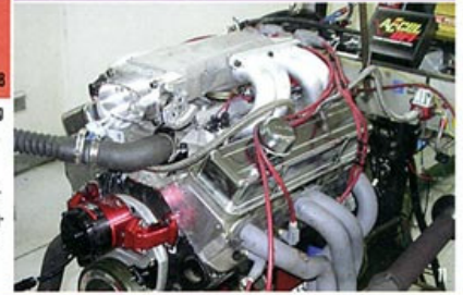
88 08 Despite their humble beginnings, the factory TPI base manifold and plenum can be made to flow better by treating them to Extrude-Hone porting. Add a set of big-tube runners (from TPIS, for instance) and you have the makings of a serious TPI system. 09 The Extrude-Hone process forces abrasive media through the ports, removing material to improve flow. The trademark wall finish is ultra smooth. The limiting factor in porting the factory base manifold is actually the size of the tubular runners. 10 We combined the Extrude-Hone ported base and plenum with a set of TPIS big-tube runners and 52mm throttle body. 11 The Extrude-Hone ported combination upped the peak power output to 451 hp, while the torque curve swelled to a whopping 534 lb-ft.
